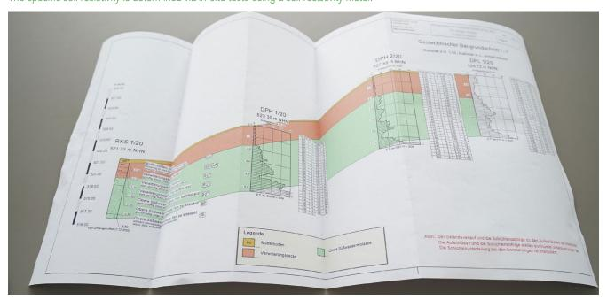
You and your structural engineer will receive a detailed report from BauGrund Süd. This includes a detailed description and assessment of the subsoil, the soil properties, the optimal ramming depth of the steel profile and the corrosion resistance.
