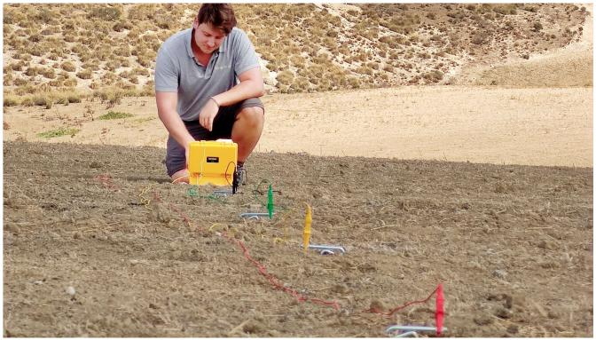
The specific soil resistivity is determined via in-situ tests using a soil resistivity meter.
