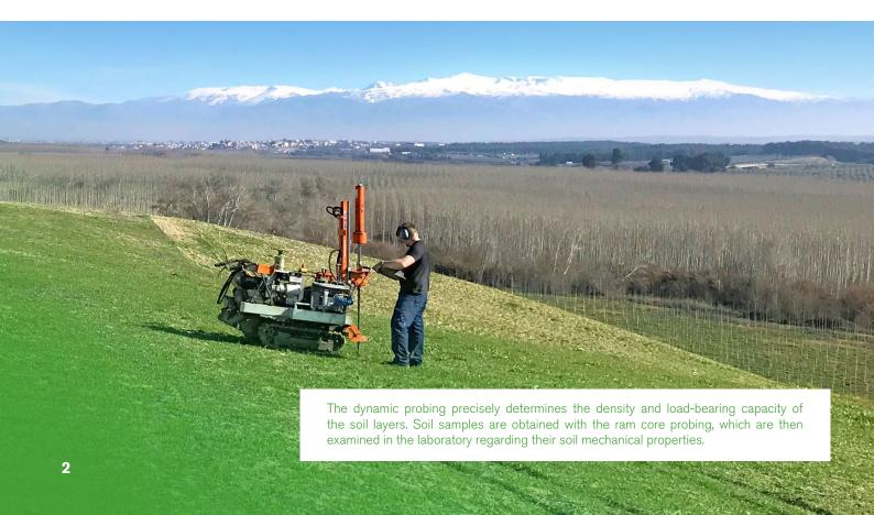
Soil samples are useful to accurately determine the geotechnical properties. We evaluate the soil at the study area and our geologists determine the mechanical and physical properties of the soil in our in-house laboratory. In addition, the corrosion probability of the soils is analyzed, which is decisive for coatings that may be required for the steel profiles.
